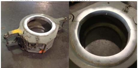
A VISUAL AND MAGNETIC PARTICLE INSPECTION WAS COMPLETED ON THE ABOVE MENTIONED EQUIPMENT. NO FLAWS WERE FOUND AT THE TIME OF THE FINAL INSPECTION.
