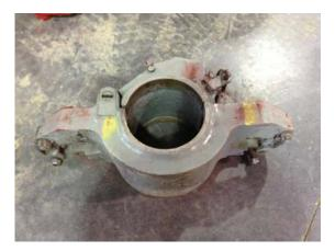
A VISUAL AND MAGNETIC PARTICLE INSPECTION WAS COMPLETED ON THE ABOVE MENTIONED EQUIPMENT. NO FLAWS WERE FOUND AT THE TIME OF THE FINAL INSPECTION.
